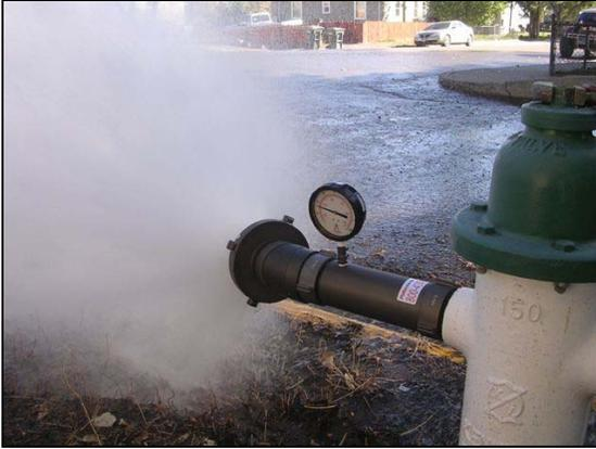
**FIELD HYDRANT FLOW TEST FOR
